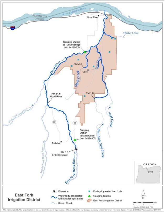
Figure 4-5. Waterbodies associated with District operations and locations of streamflow gaging stations.
