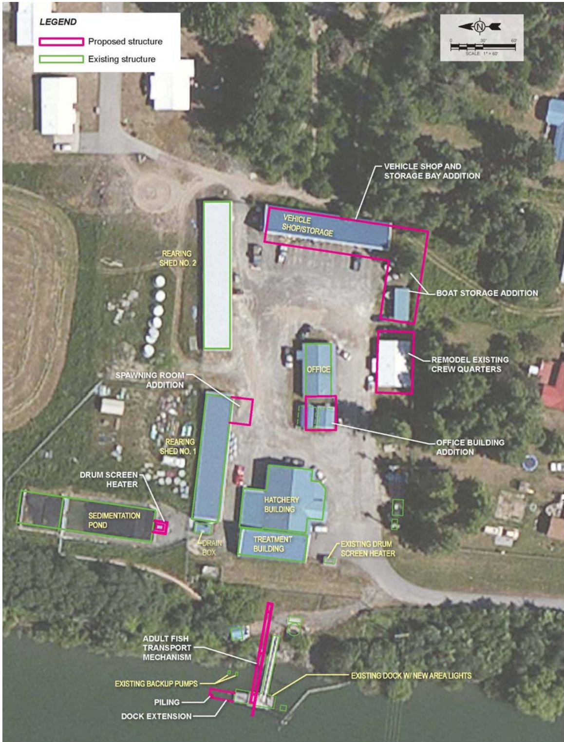
Figure 2-2: Proposed Tribal Hatchery Upgrades
