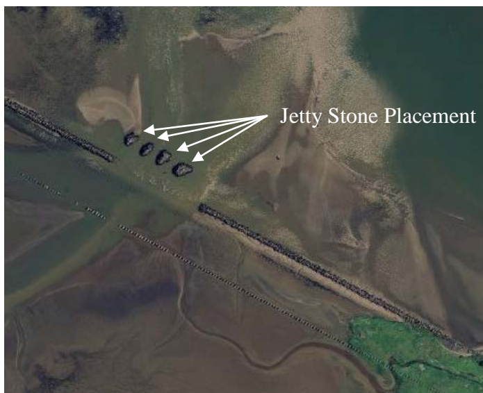
Figure 7 –Stone Piles Created from the 500-foot of Jetty Opening in 1995
