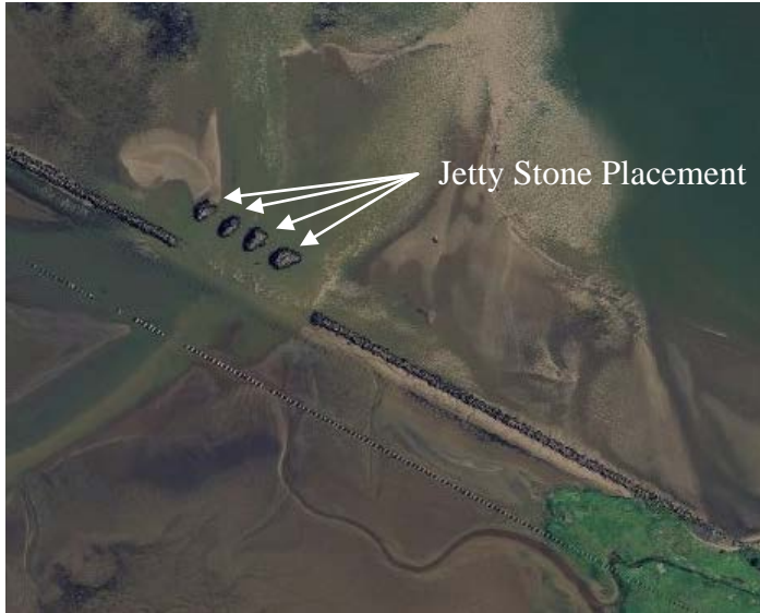
Figure 7 –Stone Piles Created from the 500-feet of Jetty Opening in 1995
