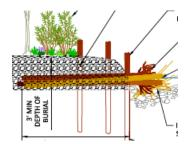
• Road Embankment Deflector Jam: Two boulders would be anchored to the same side of 30+ ft. long log (with and without rootwads) via a 1.25 inch threaded rod that is kept in place with epoxy. Steel plates and heavy hex nuts would be used to further secure the rod. These log and rock structures would be "layered" (2 layers with 5 and 3 log/boulder structures) along the road embankment.
