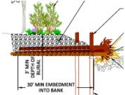
• *Buried Jam with Bumper Logs*: 3-7 Horizontal logs (2 bumper and 3-7 with rootwad attached) embedded 30+ ft. into bank and 3-7 vertical snags embedded 20+ ft. into river bed would be installed in an excavated trench (3 ft. min depth).
