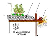
• *Large Buried Jam*: 4-7 Horizontal logs (1 bumper and 2-7 with rootwad attached) embedded 30+ ft. into bank and 3-7 vertical snags embedded 20+ ft. into river bed would be installed in excavated trench (3 ft. min depth).
