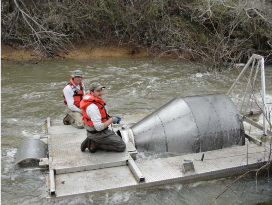
Figure 8. Example of a rotary screw trap
