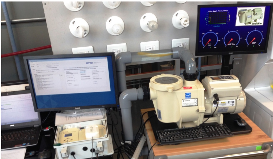
PRI Simulator Software (Top Left), Pentair Demand Response Controller (Bottom Left) and the Pentair IntelliFlo Pool pump demo with computer monitor displaying Flow rate, watts and pressure.
