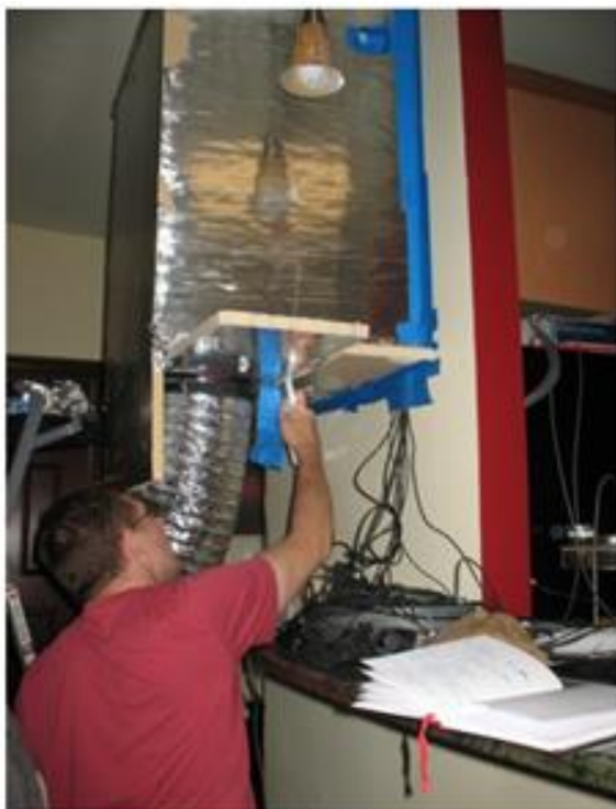
Figure 6. Example setup using a temporary rigid plenum for air flow testing of a non-ducted mini-split indoor unit
