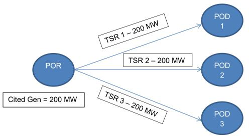
POR – Point of Receipt Cited Gen – Generation Facility Capability Cited in Data Exhibits POD – Point of Delivery TSR – Transmission Service Request
